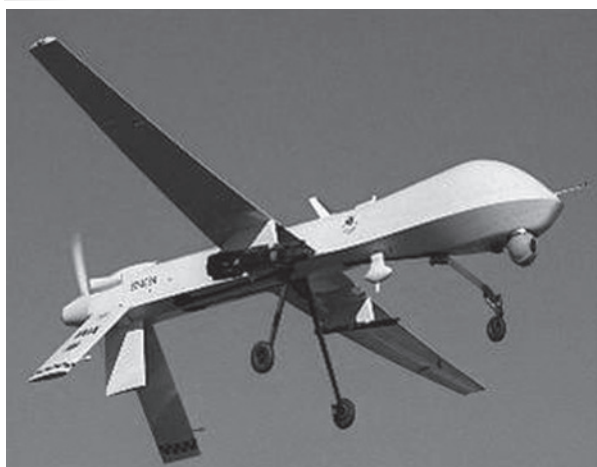
Predators strike enemy forces An MQ-1 Predator unmanned aerial vehicle is armed with an AGM-114 Hellfire missile. The Predator's primary mission is interdiction and conducting armed reconnaissance against critical, perishable targets. (USAF photo)
