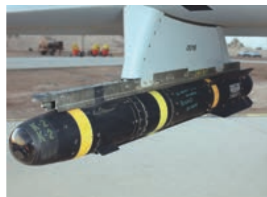
An AGM-114 Hellfire missile hung on the rail of an US Air Force MQ-1L Predator Unmanned Aerial Vehicle (UAV) is inscribed, “IN MEMORY OF HONORABLE RONALD REAGAN.”
